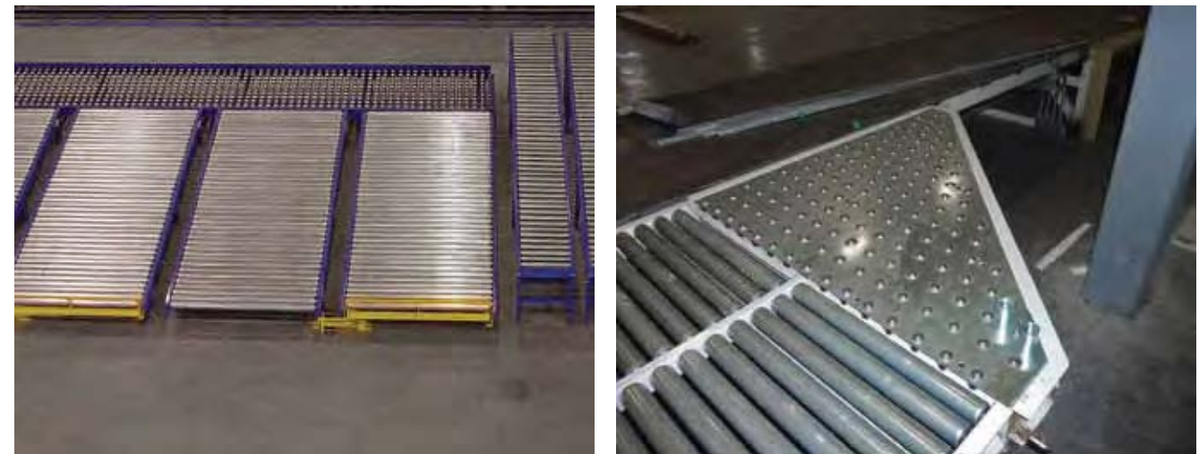
Ball transfer units enhance conveyor systems by allowing material to move omni-directionally with little effort. Photos courtesy of Ashland Conveyor, Ashland, OH
